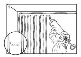
1. Cut the cartridge at the second nozzle and then apply Fix ALL Crystal glue in tight cords. Mark a perimeter the size of the cut panel to ensure a seal at the joints.
