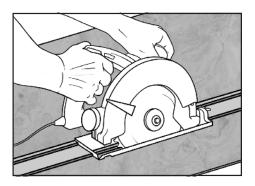
Beforehand, mark the cutting line with a pencil on painting tape on the stone side. Cut using a circular saw fitted with a carbide blade or a diamond disc. Use a guide.
