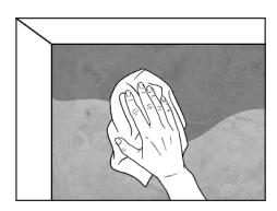
Dampen a dry cloth with Akemi water repellent product and protect the stone evenly. The water repellent will remove excess glue at the same time (within 10 minutes after installation). 20 minutes later: remove the excess product with a clean cloth.
