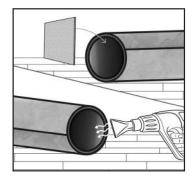
**2.** Let the sheet relax and continue to heat it flat on the resin side. Before proceeding with the cutting and installation, the stone sheet must be completely flat.
