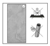
**4.** Once the stone sheet is flattened, make your cuts if necessary. **Caution,** do not put heavy weights on the stone sheet and do not cut it while it is in the form of a roll
