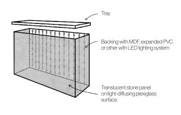
For an application on a bar or in wall formwork, place the lighting on the rear side using an LED curtain, for example. Place the translucent stone panel on the other 3 transparent sides.
