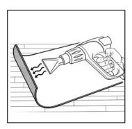
**3.** In order to optimally relax the resin, place a cardboard support at one end and heat with a thermal stripper the inside of the roll at the other end. Let it heat for 3 min.
