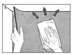
**3.** Position the panel. Using a clean cloth adjust and then smooth out the entire surface to allow adhesion to the glue.
